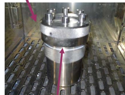
The reaction furnace and hydrothermal vessel
