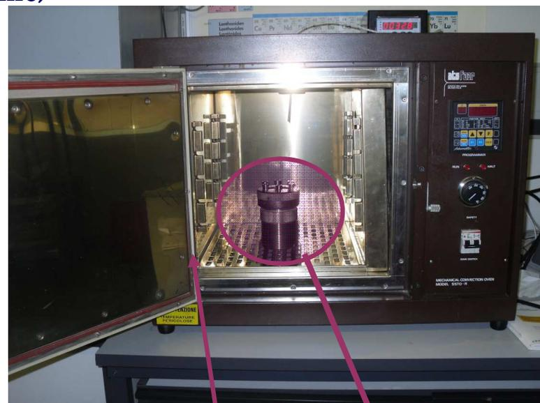
The hydrothermal treatments were conducted in the temperature range 180-220°C for 4-48h.
