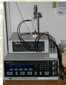
E4991A RF Impedance/Material Analyzer
